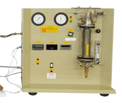
This is a closed loop unit supplied as two complimentary modules containing the certified electric boiler, pump, impulse turbine and condenser. The unit allows students to identify and compare theoretical maximum efficiencies with actual overall results.
