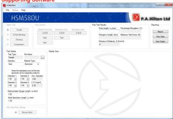
The system displays and captures data relating to elongation, extension and applied force
