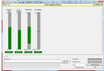
The Hilton Data Logging software supplied as standard with the HBC100A package allows the logger to be disconnected from the HB100 and used together with most standard transducers as a standalone computer data logger for the instrumentation and monitoring of existing laboratory equipment using locally sourced industrial transducers.
